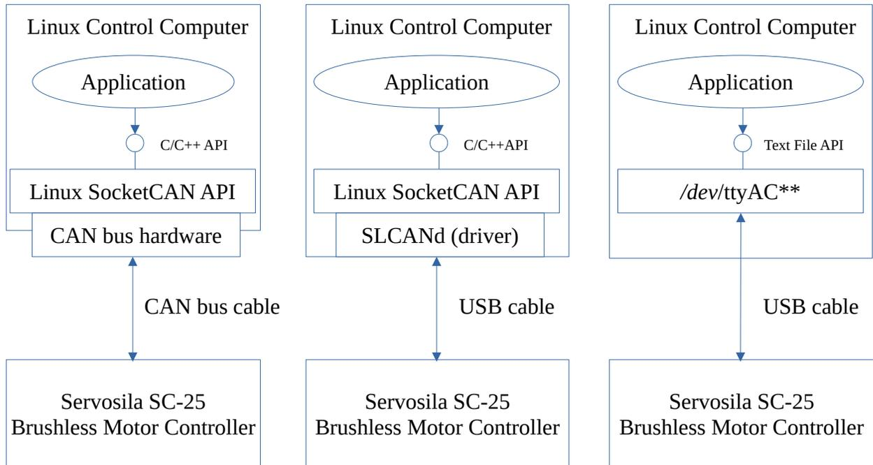
Linux SocketCAN API can be used to develop software that sends commands to SERVOSILA controllers or receives telemetry back from the controllers.
