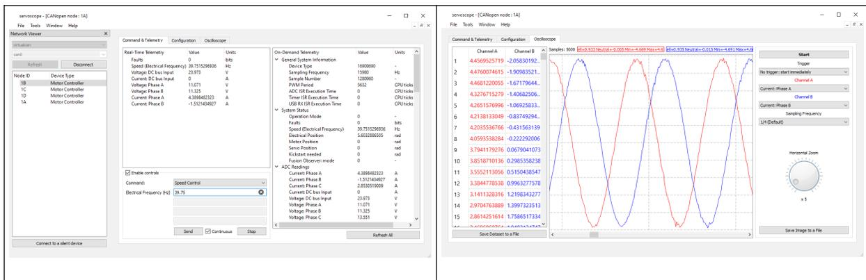
The application runs on Windows 10/8 or Linux including the popular distributions of Debian and Linux. No drivers need to be installed on either of the platforms to run the tool. The tool connects to Servosila controllers via CANbus or USB interfaces.
