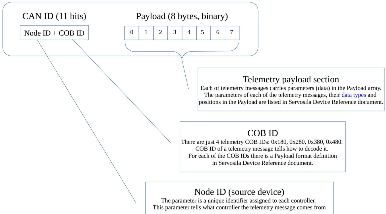
See sample C++ projects `slcan-telemetry` and `canbus-telemetry` for an example of how to receive and decode a telemetry message coming from a Servosila SC-25 Brushless Motor Controllers.
