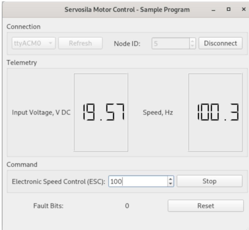
*Figure 1: Screenshot of MotorControlGUI, an example project written in C++ with Qt library. The sample program runs on both Windows and Linux. The source code of the application is freely available for modification, reuse or distribution.*
