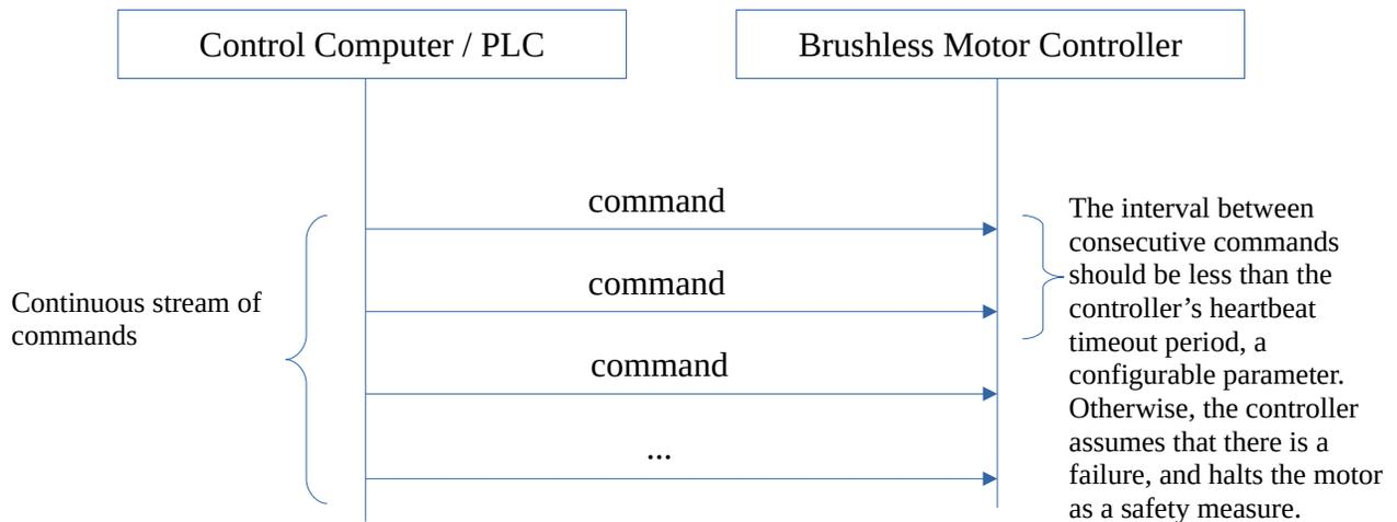
The control computer is expected to *continuously* send commands<sup>2</sup> to each of the Servosila SC25 Brushless Motor Controllers on the network. If such a continuous stream of commands suddenly stops coming to a motor controller, the controller assumes that there is a network fault or a failure in the parent control system. In such a case, the controller stops its motor as a safety measure, and might enable a brake function depending on configuration settings.
