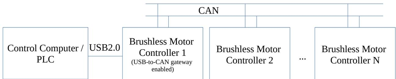
In this network architecture, it is allowed to connect third-party CAN devices to the network of brushless motor controllers. In such a case, the control computer communicates to the third-party devices via the USB-to-CAN gateway function in the same way as it communicates to the brushless motor controllers themselves.
