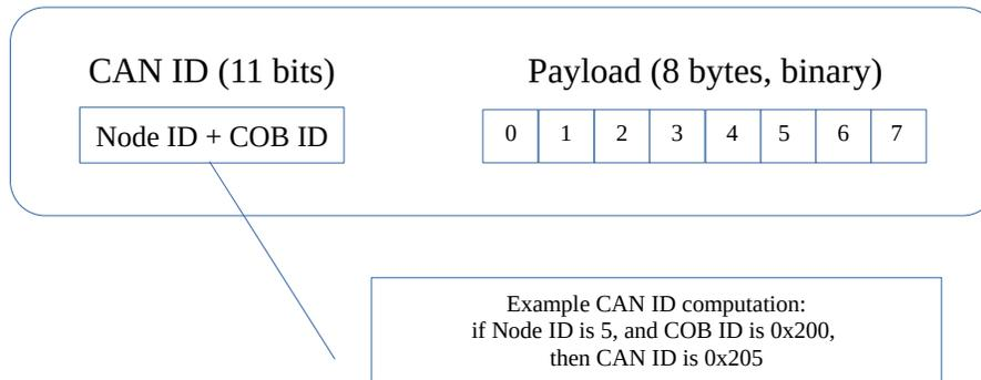
All types of messages consist of just two components, a **CAN ID** and a binary **Payload**.
