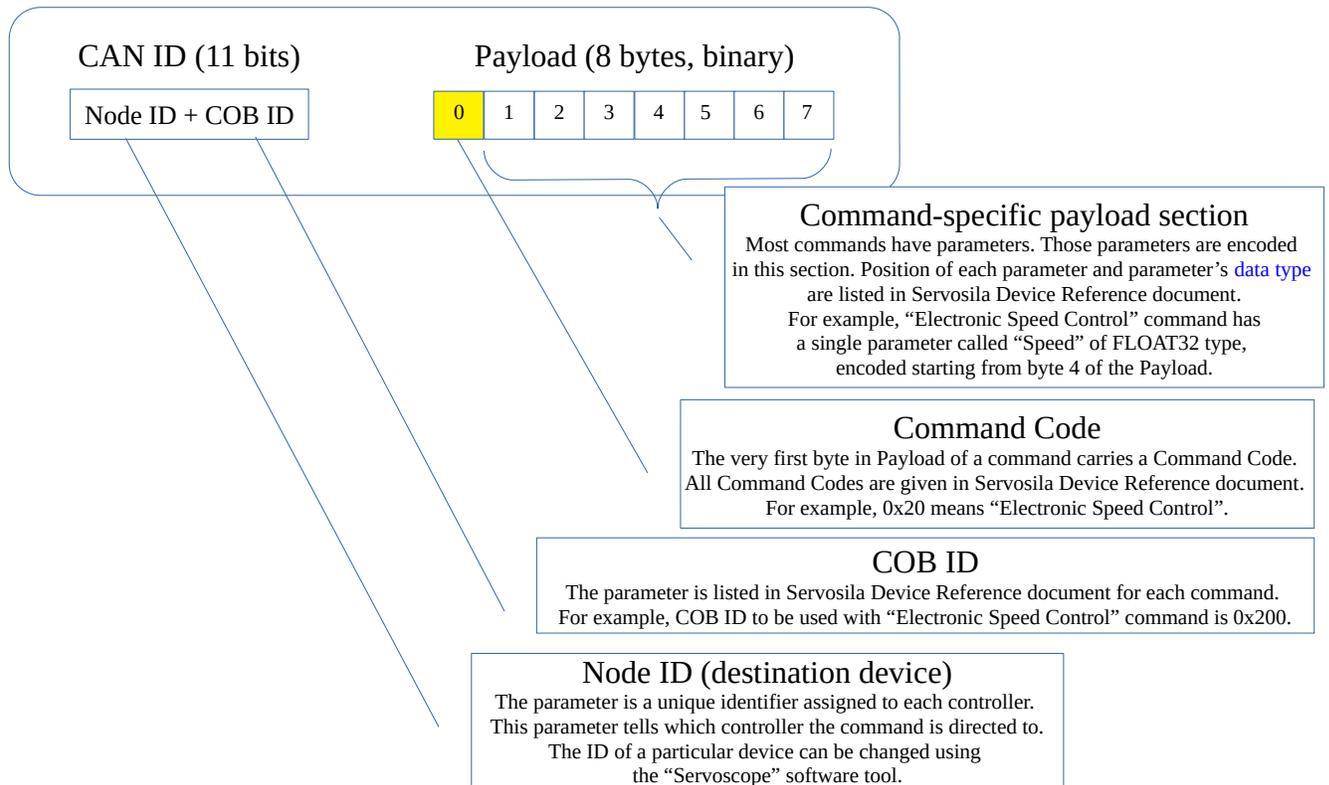
See sample C++ projects `slcan-esc-command` and `canbus-esc-command` for details on how to encode and send out a command to a Servosila SC-25 Brushless Motor Controller.
