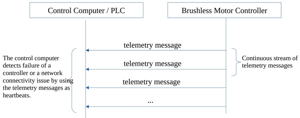
Servosila SC25 Brushless Motor Controllers continuously (periodically) send telemetry messages<sup>3</sup> back to a parent control system. The interval between telemetry messages is configured via the “Servoscope” software tool. The telemetry messages are sent asynchronously, and are not synchronized to commands or requests coming from a control computer.
