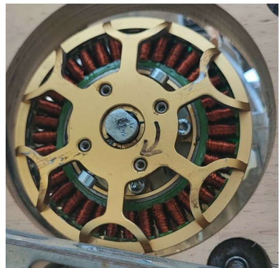
Figure 4: A brushless electric motor that acts as a stator and generator
